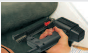
Using the MET 4000 for fixing stretched carpets
