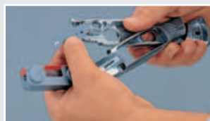
Insertion of the new blade.
